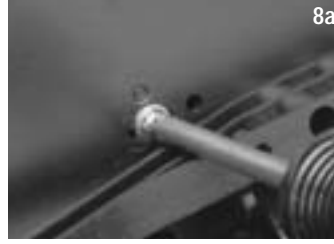
8a Set the carb linkage bell crank post assembly back onto the chassis (keying the post into the appropriate holes) and secure it with the 3x10WM screw.
