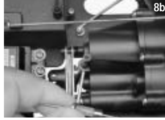
8b Insert the brake lever into the brake cam and tighten the 3x3GS. Install the air filter back on the carburetor. This completes the 2-speed installation.
